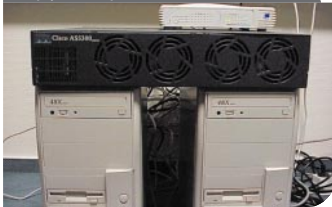
The physical setup: 2 PCs and 1 Cisco access router
